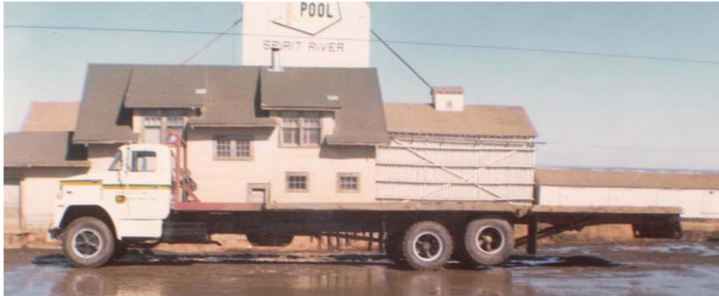
You are looking at Expo II a 1975 CT800 Dodge truck with hyd tag axle, hyd rear ramp, & hyd winch. The main deck is 22' long & the tail ramp is 13' long total deck 35' . We have a picture of Dave loading a old Steam Engine on Expo to haul it to the museum, This was Daves pride & joy next to his original 1940 Fargo. In the back ground the first building was the S.R NAR railway station. The elevator in the back ground is the Alberta Wheat Pool.
