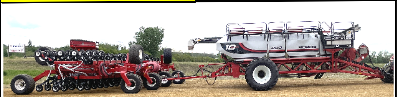
10 Series 915720 820 bu, 4 Tanks 80 bu, 250,bu, 135 bu, 355bu, + Tank Load Cells dual fans Top ConXD + monitor 5m3397 duals 4-900/60R42 Convey-All Conveyor Sect Control + 70' Quantum 9m5332 Air Drill 12" Spacing paired row dbl shoot 3 Row Packer Control, 820 bu Cart $545,000 +70' Quantum $450,000 = msrp $995,000 cod $895,000
